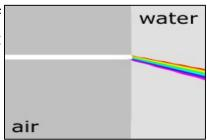
When a ray of sunlight enters a raindrop, it bends (refracts). The light then strikes the back of the raindrop, where some of the light passes through and some is reflected. As the light exits the raindrop, it is refracted again. The angle at which the light emerges depends on the wavelength of light. This path is illustrated in the small box below, where only the bending of two wavelengths (blue and red) are shown.
